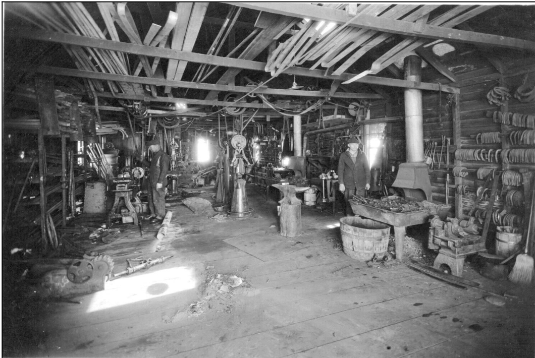
Interior of Herman Martin’s new Blacksmith shop circa 1920s, generally as it appeared when Cliff took over in November 1934 upon the death of his father. In the center is the trip hammer, the anvil, and the old forge with chimney. Note to the right on the wall is a selection of horseshoes. Grandpa Martin shod horses, but Cliff never did. The two men in the picture might be Kink near the forge and Herman left near grinder.
